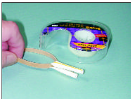
A piece of soda straw is bent over and taped to a #64 rubber band.
