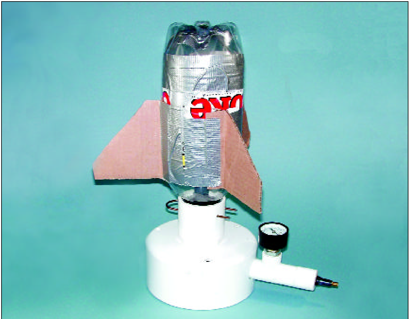
Pop Bottle Rocket Mounted On Versey Launcher
